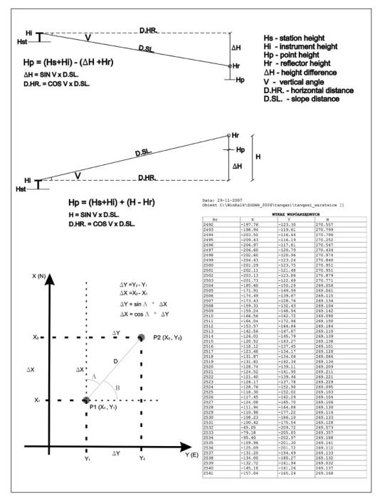
Fig. 1. Basic topographical measurement scheme (based on the author's original documentation from the Tanqasi cemetery, 2006)
